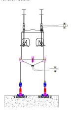
Compression scale, on concrete floor:
