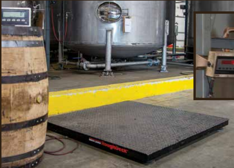
RoughDeck floor scales weigh barrels and totes while 320IS indicators display weights at various stages of bourbon production. Intrinsically-safe equipment is installed throughout the distillery.
